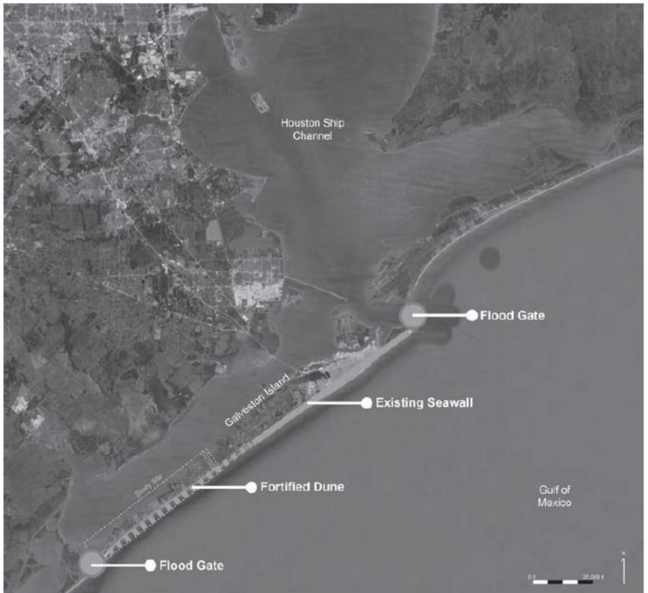
Figure 1. The Ike Dike's potential storm surge structural infrastructure components; Galveston Island's proposed coastal spine is designed to protect the Houston-Galveston Metropolitan Statistical Area (H-G MSA) from a 10,000 year flood.
