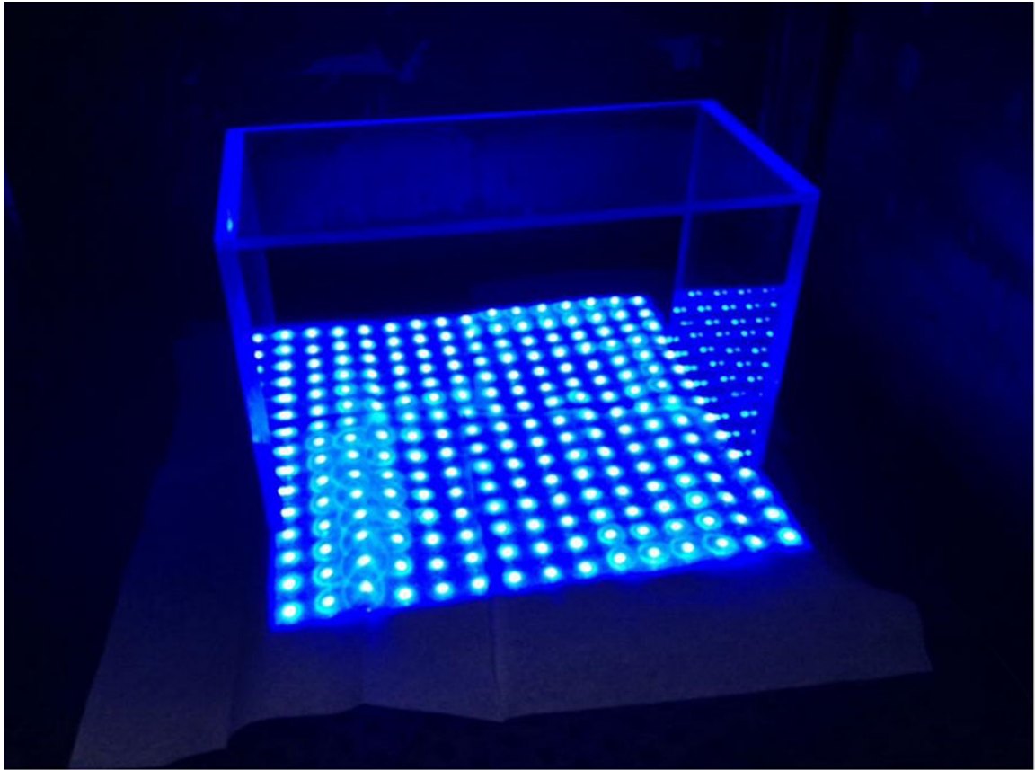
Fig. 1. The light-emitting diode-based blue light source used in the current study. The rack above the light panel maintains the desired distance between the cell culture plates and the blue light source. The light intensity was measured by Dr. Meter LX1010B 100,000 Light Meter with LCD Display (Hisgadget Inc, US) as 2500 lux.
