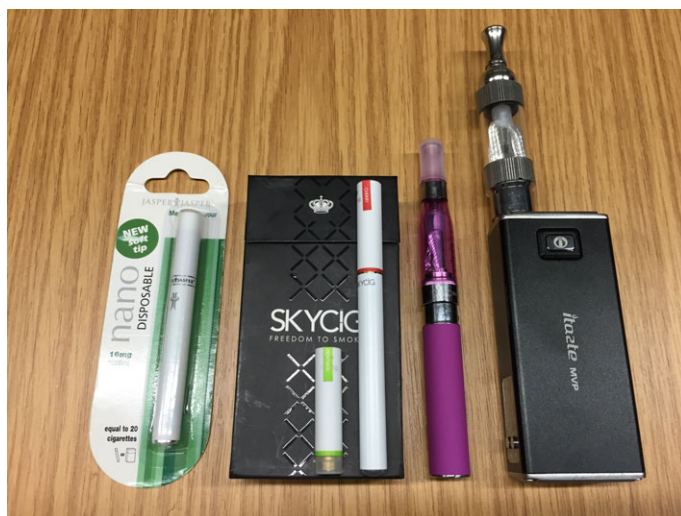
Figure 1 E-cigarette props used in interviews. From left to right: disposable cigalike, reusable cigalike with interchangeable flavours (packet contents on exterior), vapouriser, box mod.
