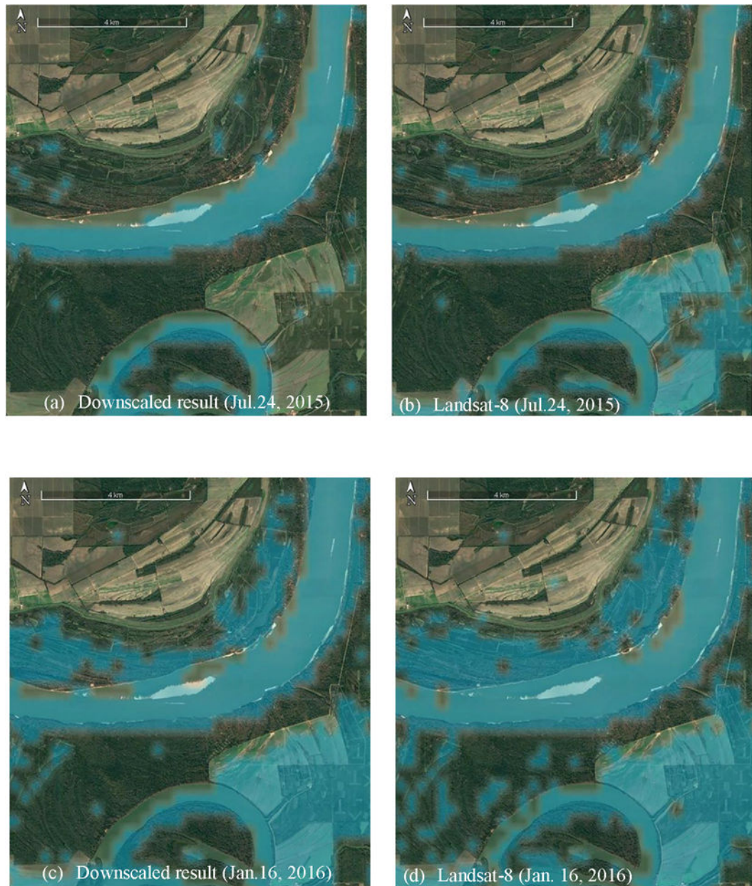
Fig.8. SMAP downscaled results (a, c) and Landsat-8 (OLI, TIRS) (b, d) classifications of water (blue) pixels overlaid on Google Earth images (Google imagery date 12/07/2014) over a selected focus area ( 0.1^{\circ} \times 0.1^{\circ} rectangle centered at -91.55^{\circ} , 31.27^{\circ} ) within region 3 and representing respective seasonal dry and wet conditions for Jul. 24, 2015 and Jan. 16, 2016.
