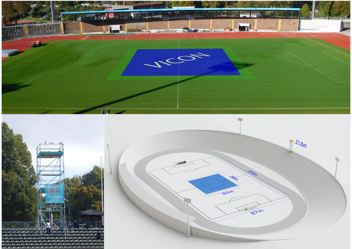
Fig 2. Venue. (Top) VICON test location on the pitch; (bottom right) scaled 3D model of the Rosenaustadion Augsburg. VICON area (blue), VID camera position (orange) at 21.6 m height and 82.0 m distance from the center spot. Pitch size: 105.0 x 67.0 m; (bottom left) additional camera platform.
