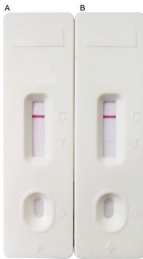
Figure 5. Results of PP14-based lateral flow assay. (A) A total of 0.005 \mu\text{g/ml} PP14 recombinant protein was added. The strip was negative. (B) A total of 0.008 \mu\text{g/ml} PP14 recombinant protein was added. The strip was positive. PP14, placental protein 14; C, control line; T, test line; S, sample well.
