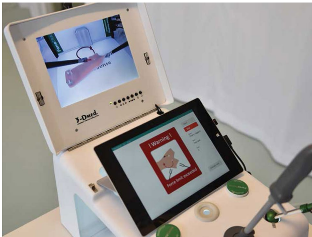
Fig. 4 Instant force feedback system shown on tablet
