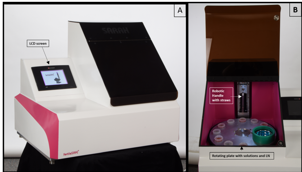
Fig. 1 Two pictures of the Sarah device. a The closed device with its LCD screen and b the open device showing the rotating metal plate with the solutions and LN container as well as the robotic handle with the straws
