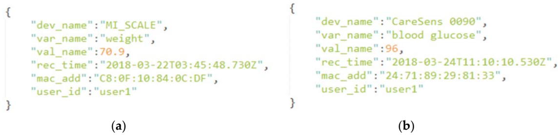
Figure 3. An example of user weight (a) and user blood glucose (BG) (b) sensor data in the NoSQL MongoDB.
