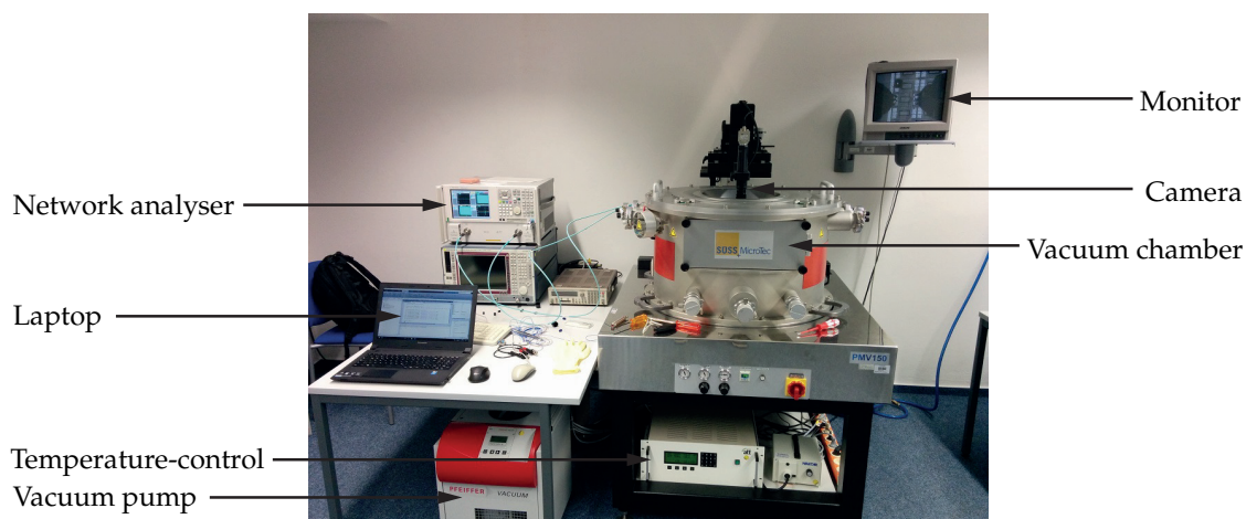
Figure 8. Measurement setup for the investigation of the temperature dependent RF behaviour of MEMS resonators. The setup consists of the vacuum chamber PMV150 (Süss MicroTec), the vacuum-pump station TSH 261 (Pfeiffer Vacuum) providing a chamber pressure of approximately 100 Pa, the temperature-control unit P150 (Advanced Temperature Test Systems) covering a temperature range from -40 °C to 150 °C, a camera with microscope and monitor, the network analyser PNA-L N5230A (Keysight Technologie, Santa Rosa, CA, USA), and a laptop for the evaluation with MATLAB.
