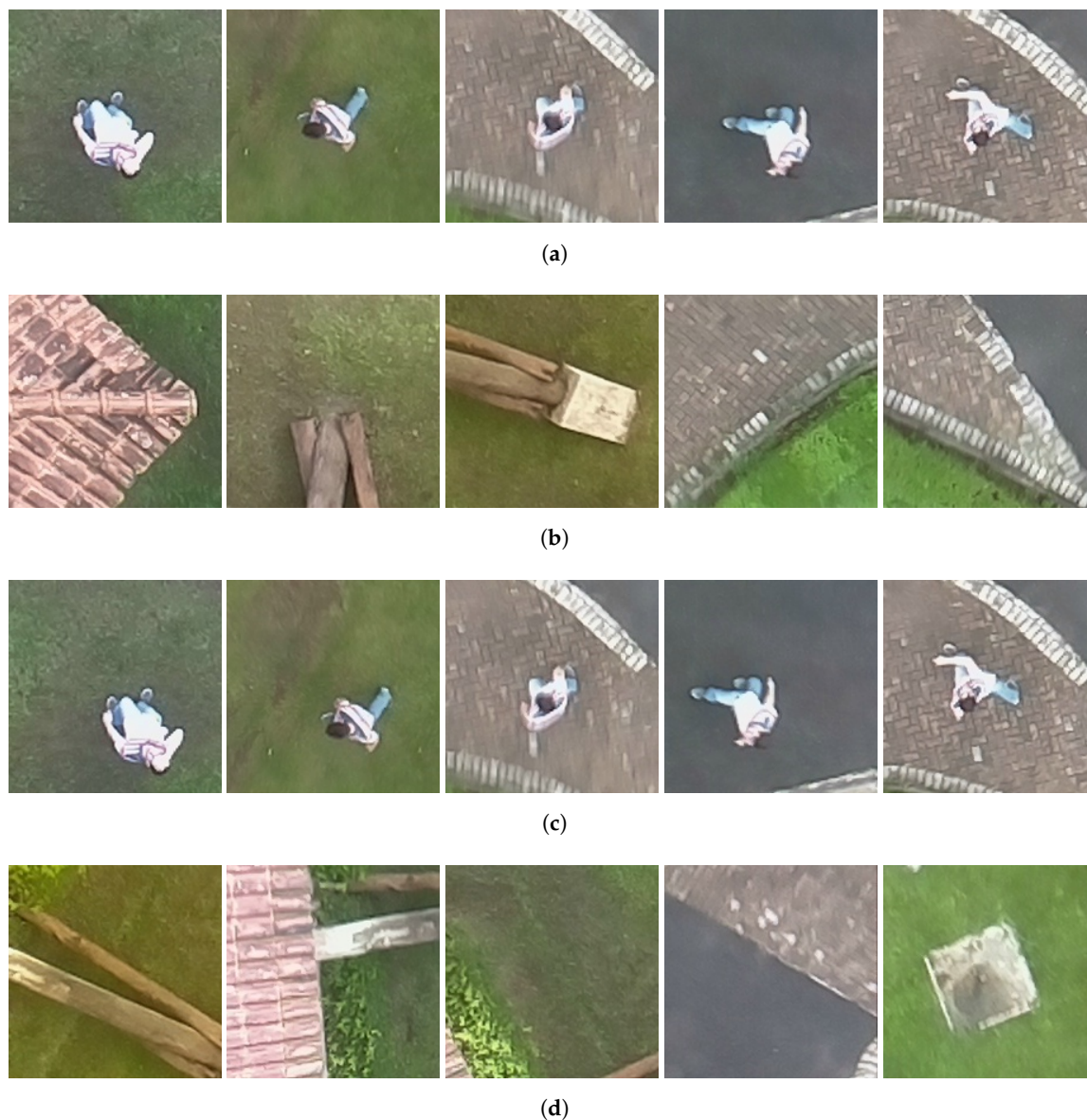
Figure 13. Samples of ROI: (a) positive and (b) negative samples extracted with saliency map; (c) positive and (d) negative extracted with thermal image processing.
