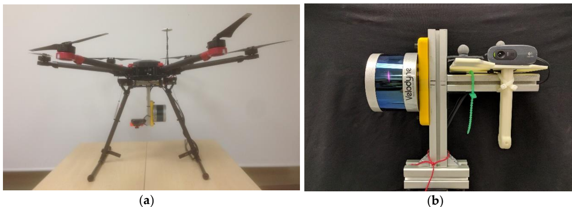
Figure 11. Hardware Prototypes: (a) early prototype UAV hexacopter deploying the sensor setup considered in this work; (b) hand-held sensor rigid body for experimentation in flight-denied areas (indoor laboratories, etc . . . ).
