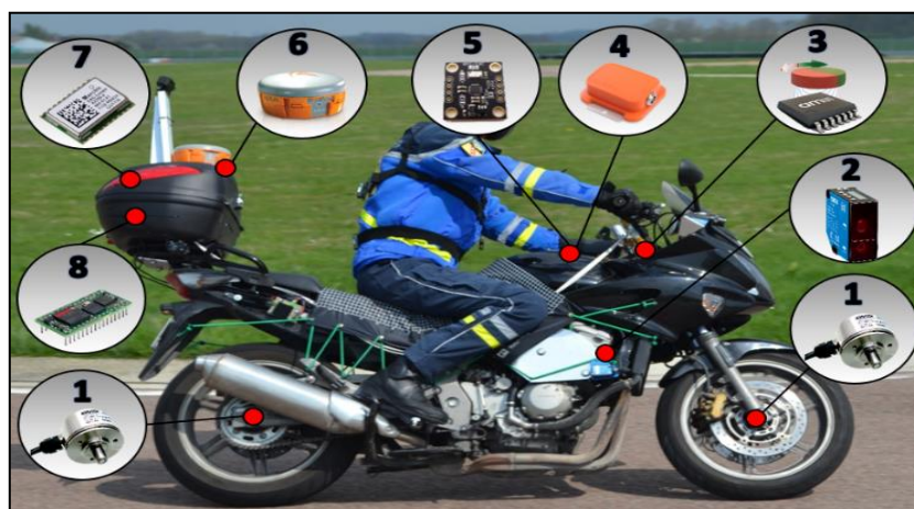
Figure 1. The ANR team instrumented motorcycle.
