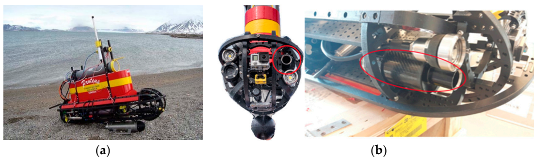
Figure 5. (a) PROTEUS vehicle; (b) front and side view of PROTEUS (circle shows ArLoC installed on board).
