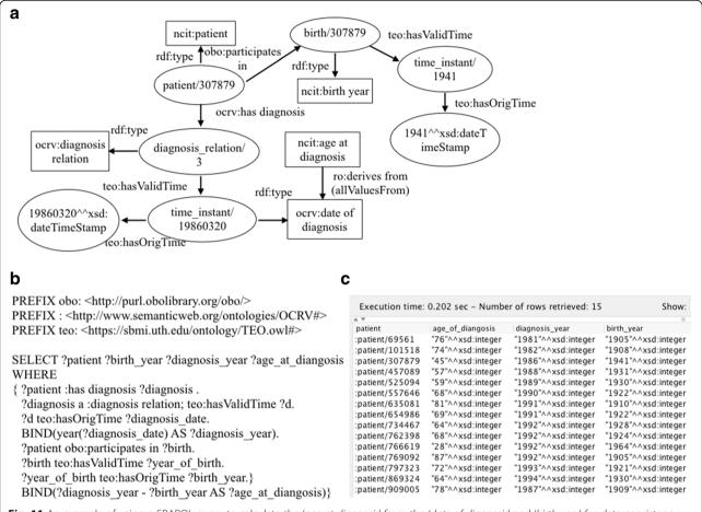
**Fig. 11** An example of using a SPARQL query to calculate the 'age at diagnosis' from the 'date of diagnosis' and 'birth year' for data consistency checks, where (a) shows a graphical representation, (b) is the SPARQL query, and (c) shows the query results
