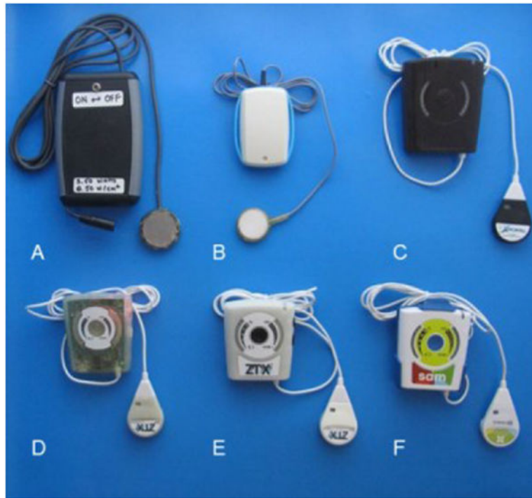
Figure 1: (a-f) Depictions of design iterations of portable, wearable device design, progressing from initial prototype towards final design.
