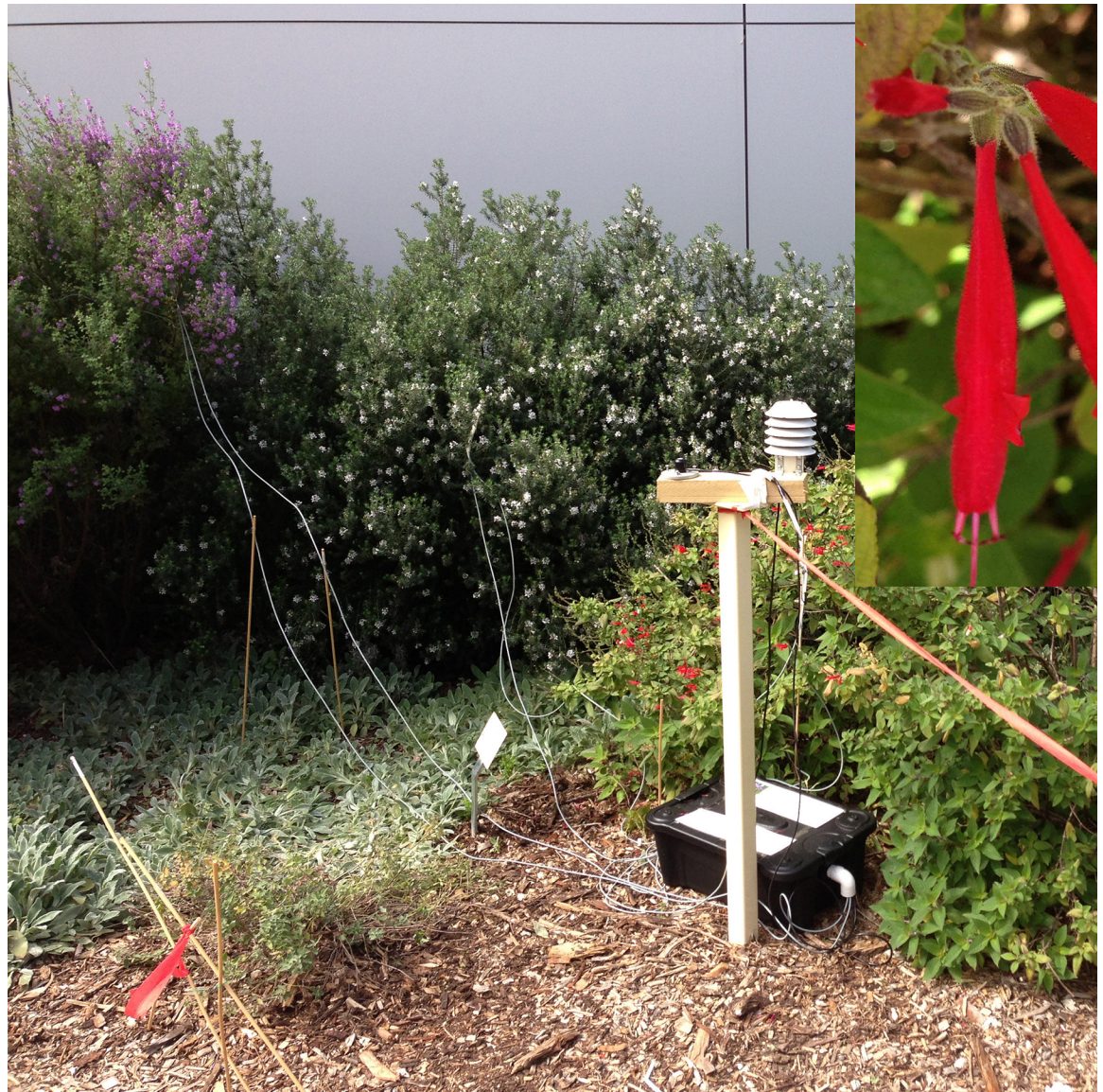
Fig 2. Equipment set up in the field to collect flower temperature readings. Inset shows the TSM sensor attached to a petal surface.
