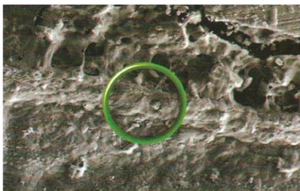
Figure 2. Ion-exchange interfacial layer formed between glass-ionomer cement (Fuji IX) and a natural tooth over five years.
