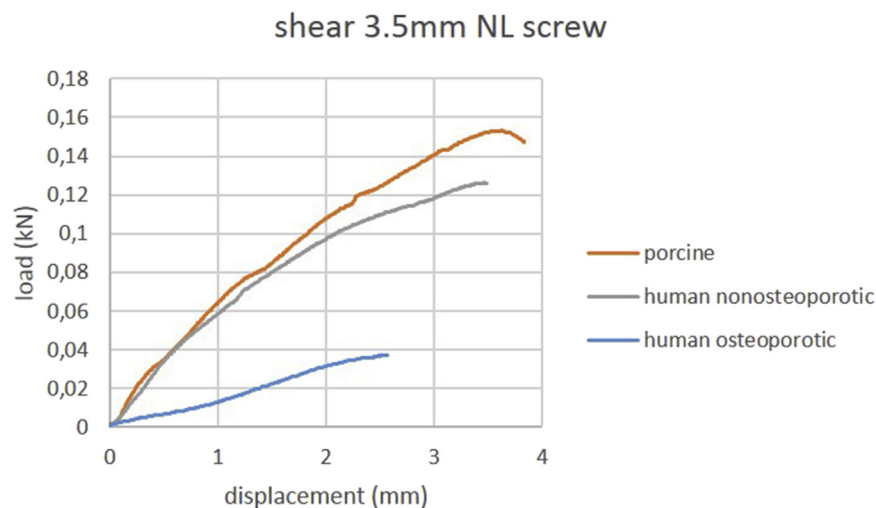
Figure 5 Load-displacement curves of shear testing using 3.5 mm nonlocking screws. Curves of one representative specimen per group are shown. NL = nonlocking
