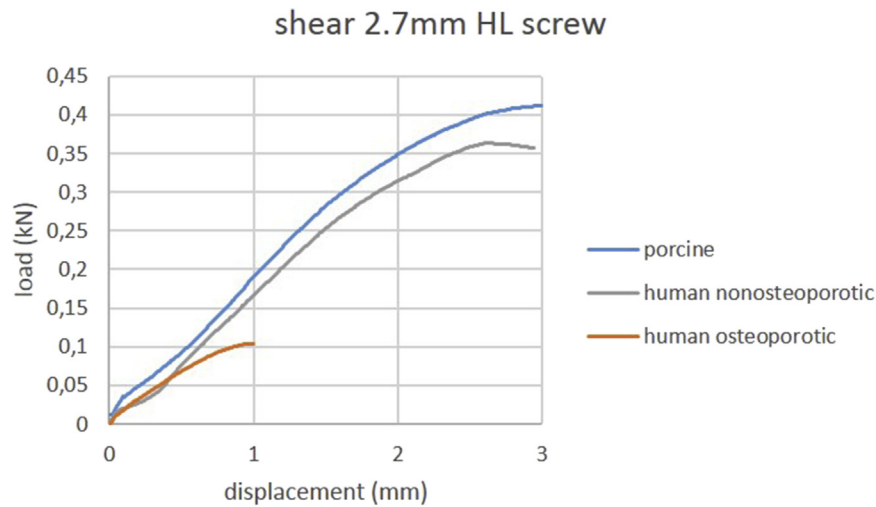
Figure 4 Load-displacement curves of shear testing using 2.7 mm head locking screws. Curves of one representative specimen per group are shown. HL = head locking.
