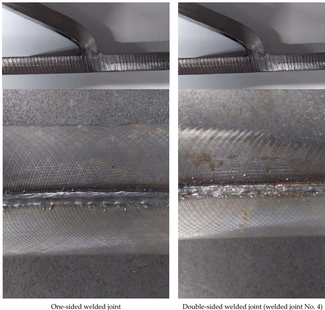
Figure 12. View of joints after bending test.
