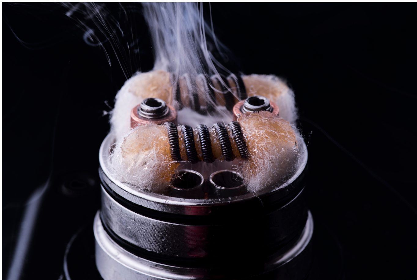
Different styles of e-cigarettes all have some form of atomizer (heating unit) and tank (or cartridge) that contains the e-liquid. The liquid is wicked from the tank into the atomizer. There it is heated by a metal coil to produce vapor. Image: © O. Bellini/Shutterstock.
