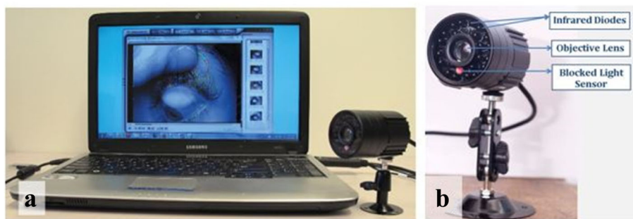
Fig. 1 a Computer - meibographer set up. b Picture of meibographer with major components labelled
