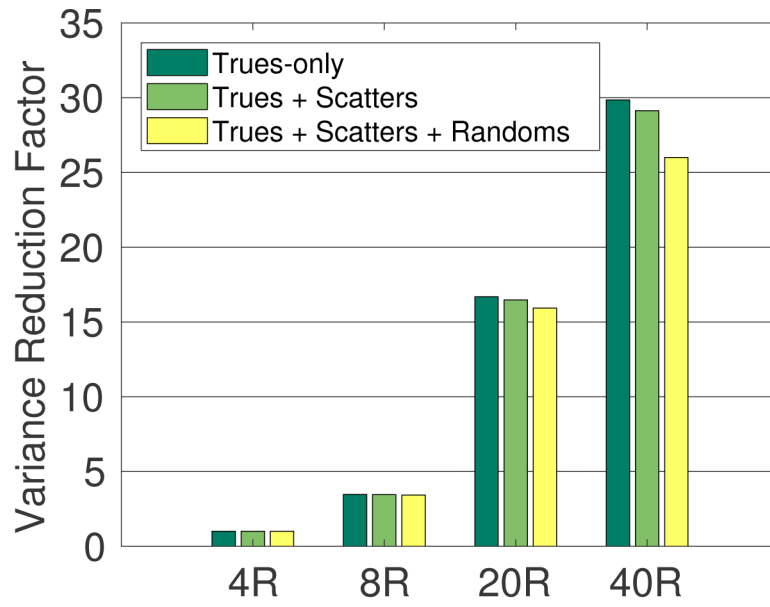
Figure 7: Variance reduction factor (CRC=0.5) of 8R, 20R, 40R scan over the 4R scan for trues-only, trues + scatters, and trues + scatters + randoms, respectively, for 10-mm ROI. All scanners are with 500 ps TOF and no DOI.
