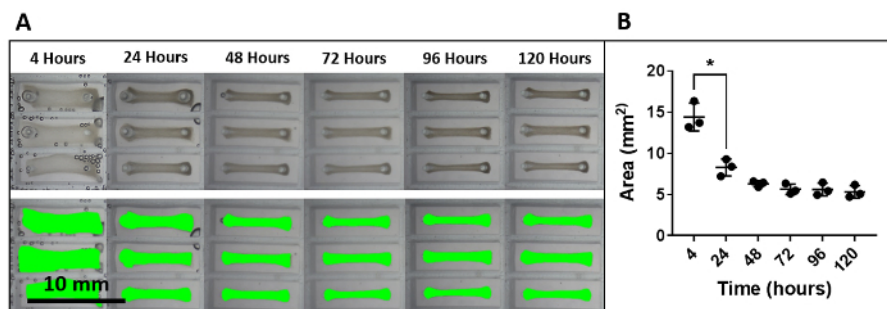
Figure 2: Construct compaction over time in culture. (A) Images of rectangular constructs prepared in triplicate compacting over time in culture. Green overlays represent masks used to calculate visible construct area for image analysis. (B) Plot of construct area (a two-dimensional metric of construct compaction) over time. Horizontal lines represent the mean values and error bars indicate the standard deviation. For all groups, n = 3 and * indicates p < 0.05 as evaluated by ANOVA. Please click here to view a larger version of this figure.
