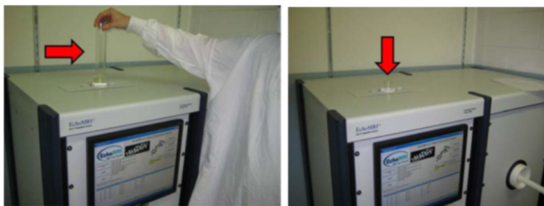
Figure 1: Correct placement of mouse COSTS and small animal specimen holder containing mice within the body composition analyzer. To perform a system test using a calibration standard (COSTS) or for scanning of mice within the small animal specimen holder, place each inside the gantry of the system. The red arrows indicate the cylinder in which the mice will be contained entering the gantry of the machine.
