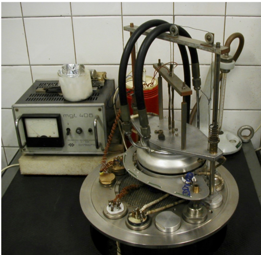
Figure 4: Apparatus for ex situ heat treatment of the as-quenched metallic glass ribbons. Please click here to view a larger version of this figure.
