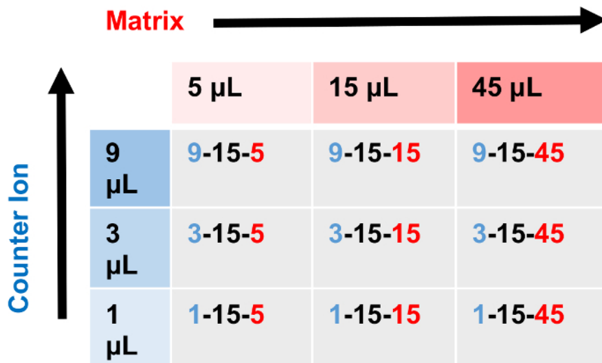
Figure 1: 3 x 3 grid for sample ratio determination. Using a 3 x 3 grid of samples, the relative concentrations of cationization agent-analyte-matrix can be systematically varied to empirically determine an optimized sample preparation. This is typically done by holding one of the three variables constant (15 µL of analyte solution) while increasing the amount of the other two (cationization agent (y-axis) and matrix (x-axis)) components by a set multiple (3-fold in the example depicted). Please click here to view a larger version of this figure.
