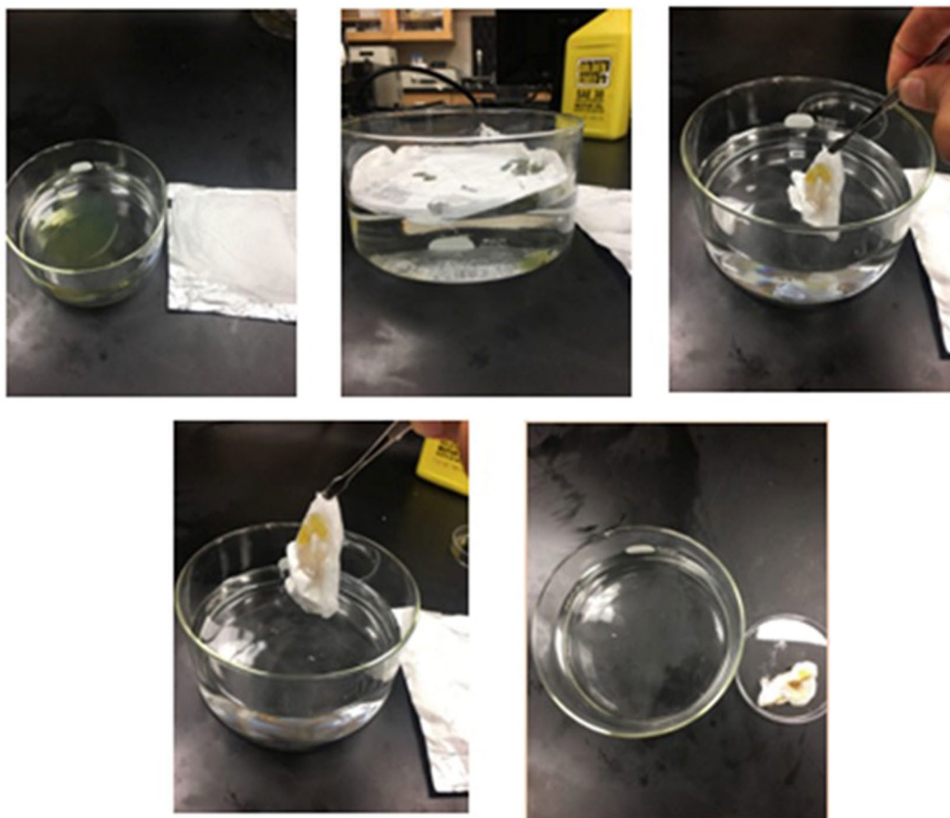
Figure 8. Testing the oil sorption efficiency of the CA electrospun mats.
