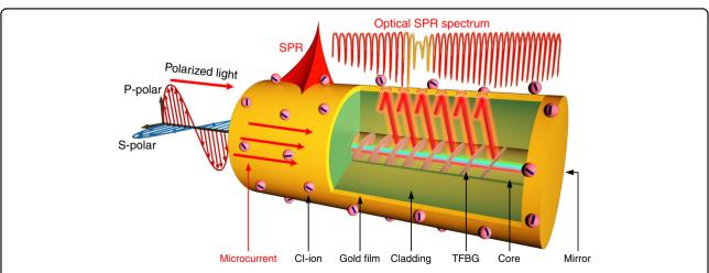
Fig. 6 Electrochemical surface-plasmon-resonance sensing principle and experimental demonstration with an gold-coated TFBG optical fiber sensor. Sketch of the configuration of a plasmonic optical fiber sensor for in situ monitoring of supercapacitors
