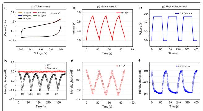
**Fig. 4 Sensor responses in the charging/discharging cycling tests. a** Five cycles of CV data and **(b)** the corresponding sensor SPR transmitted intensity; **(c, d)** same as **(a, b)** but for 3 cycles of GCD; **(e, f)** same, but for 3 cycles of GCVH
