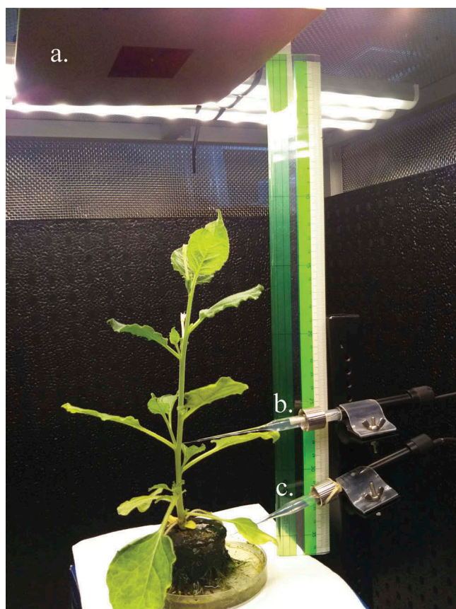
Figure 1. A representative image of Nicotiana benthamiana wildtype plant during electric potential recording. Letters a, b and c represent top hanging transmission microstrip antenna, reading glass electrode, and reference glass electrode respectively.
