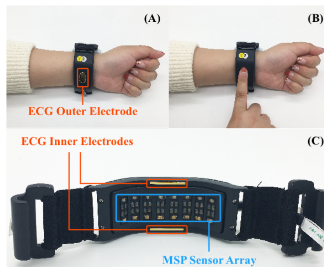
Figure 11. Snapshots of our in-house data acquisitions for ECG (A,B) and MSP (C). One wearable ECG sensor contacts the wrist of the left arm (A) and a subject must touch ECG sensors with their index finger of the right hand to acquire ECG data to measure the potential difference between left wrist and right finger (B). MSP sensor array is placed on the right wrist to measure the data (C).
