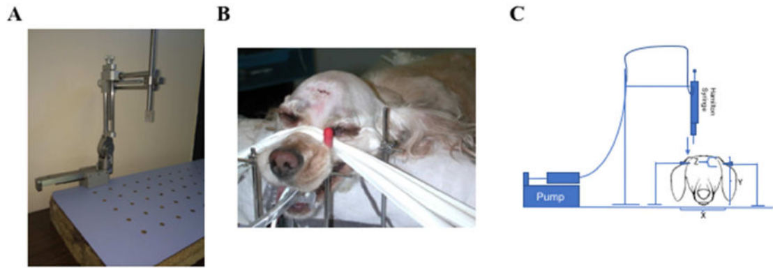
Fig. 1. Canine nanoparticle CED System. A. Stereotactic infusion system. B. Photo of dog positioned for surgery for infusion. C. Schematic representation of stereotactic catheter delivery system showing infusion pump, Hamilton syringe, reservoir, frame, and canine subject.
