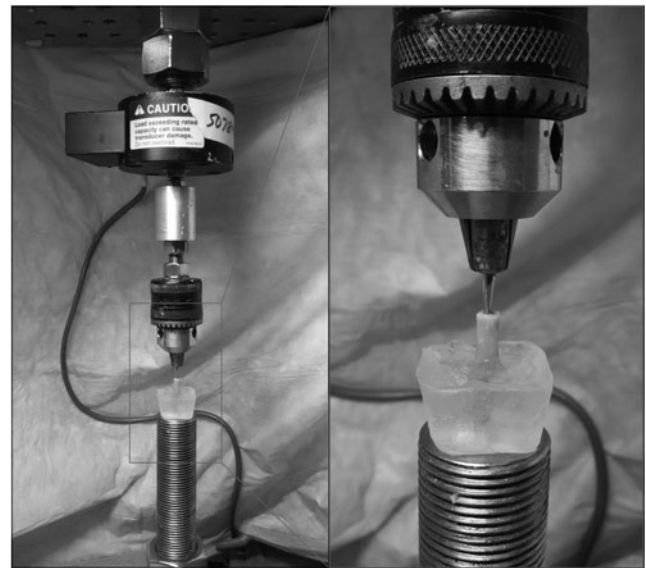
FIG. 5. Mechanical pushout fixture with potted specimen.
