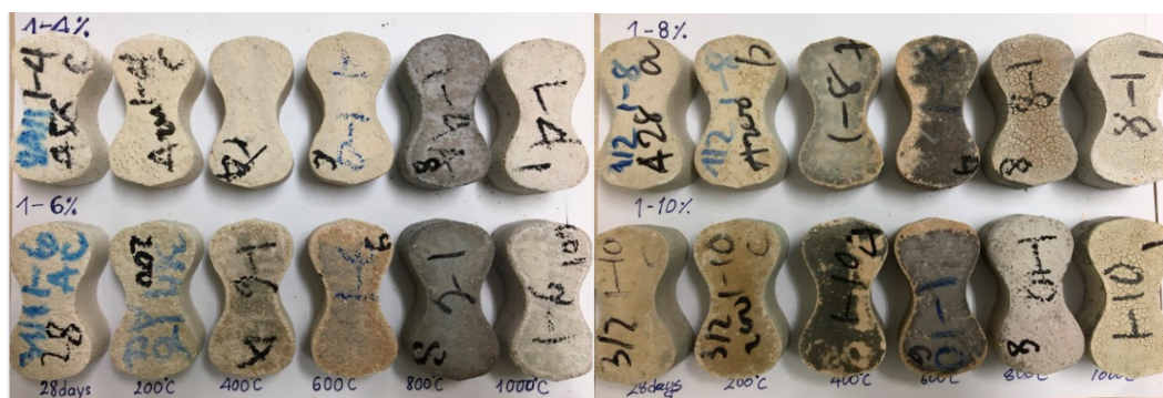
Figure 4. Photographs of AAS mortar samples activated with different concentration of Na 2 O before and after exposure to high temperatures from 200 to 1000 °C.
