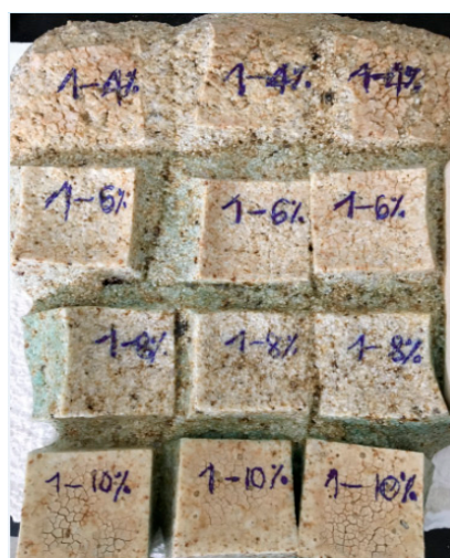
Figure 5. Photograph of AAS mortar samples after exposure to 1200 °C.
