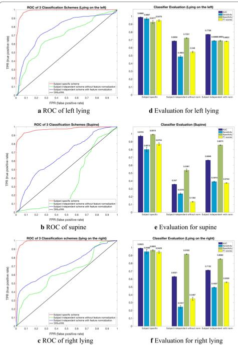
**Fig. 6** The classifier performance of three schemes. Graphs (**a–c**) are the ROC curves of three kinds of lying position. The red line represents subject specific scheme, green line represents subject independent scheme without features normalization and blue line represents subject independent scheme with features normalization. Bar charts (**d–f**) present the mean value of AUC, Sensitivity, Specificity and F1-scores of 10 experiments
