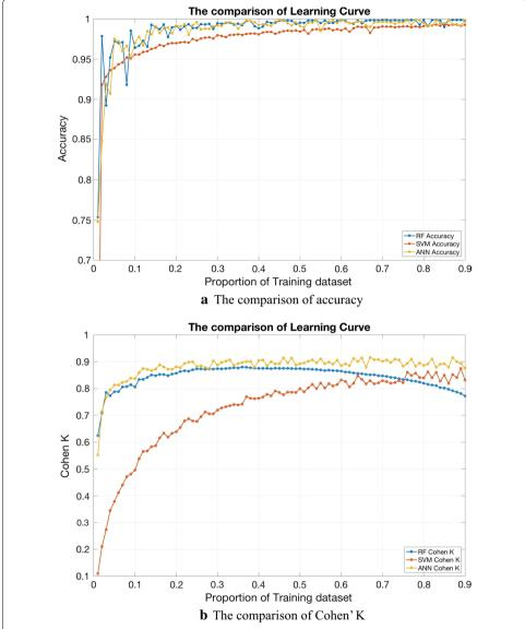
**Fig. 8** The comparison of the classification performance between RF, SVM and ANN. We can see that RM and ANN perform better than SVM, and the accuracies of RF and ANN are close. The Cohen'k of ANN is slightly higher than RF. However, the calculation of RF is much faster. Consequently, RF performs best in general
