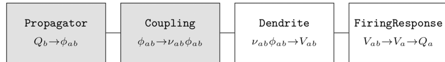
Fig 4. NFTsim classes associated with biophysical processes. This diagram illustrates the relationship of the classes in the library and the biophysical transformations they represent. Input variables are on the left, while output variables are on the right. Gray boxes are classes associated with interactions between populations, while white boxes are classes associated with internal mechanisms of a population.
