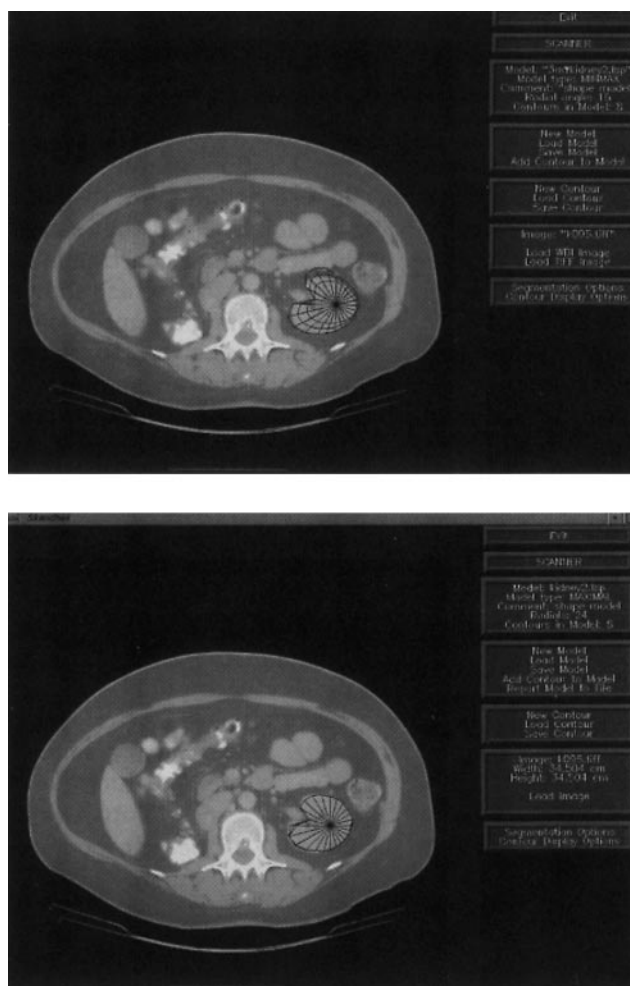
Figure 5 F-2-D, shape-based image segmentation in the Scanner program. A: Initial 2-D radial contour model after user has indicated two endpoints, and constraints have propagated to generate an initial uncertainty region delineated by the inner and outer contours, and a bestguess contour as the midpoints along the radials in the uncertainty region. B: Final stage, after all edges have been found.
