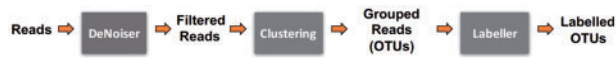
Fig. 1. A basic metagenomics pipeline. Raw sequence reads are filtered for quality during a denoising step, followed by clustering into groups (called OTUs) and a labeling of each OTU with the closest corresponding phylogenetic classification
