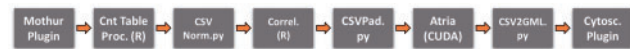
Fig. 3. Our test metagenomics pipeline, P-M16S. Note plugins have been implemented in various programming languages, and some have been generated by PluGen. File conversion plugins have been downloaded from the PluMA plugin pool
