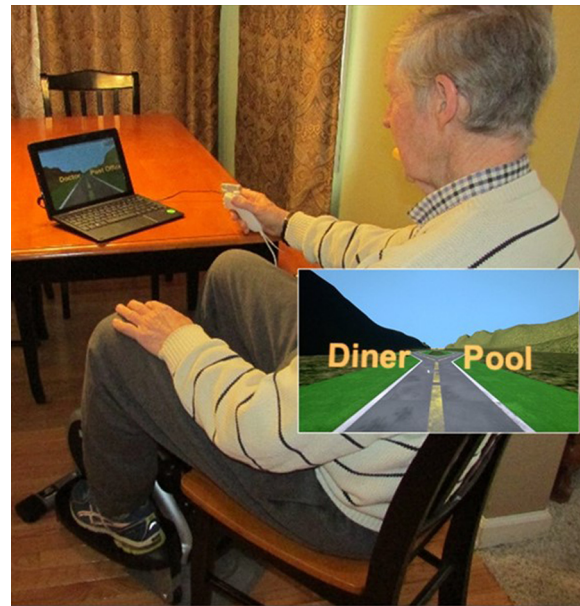
Figure 1 The interactive Physical and Cognitive Exercise System (iPACES) shown as used in-home via a portable tablet-laptop paired with a cadence monitor on an under-table elliptical and operated by a joystick equipped with a HR monitor (finger sensor).
