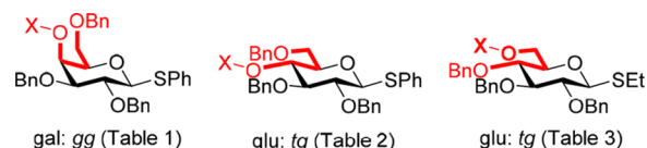
Figure 6. syn -Pentane conformations of the galacto- and glucopyranosides destabilized on replacement of a hydroxy group ( X = H ) by an ether ( X = R ).
