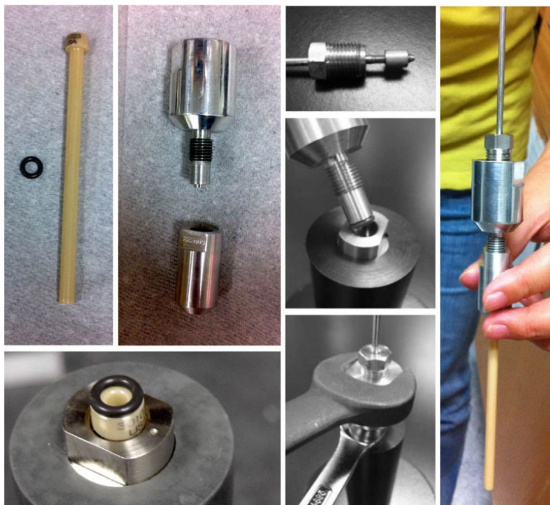
Figure 2. Assembly of NMR cell. The NMR tube and its o-ring are seated in the lower half of the metal valve and aligned using a setup tool (left). The upper half of the cell is then screwed on and iterative cycles of tightening and aligning are performed using a torque wrench set to 130 lb. in. (middle). The sealed pressure valve-NMR tube assembly is connected to a pressure generator via a tether that is screwed on to the top of the cell (right). Some photos courtesy of Daedalus Innovations LLC.
