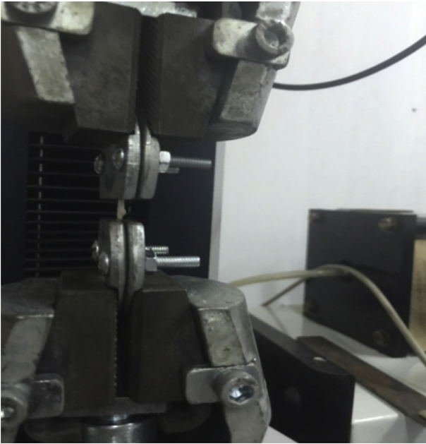
Fig. 5. Mecmesin mechanical test device and specially designed unnotched grasper jaws, which hold the tendon.
