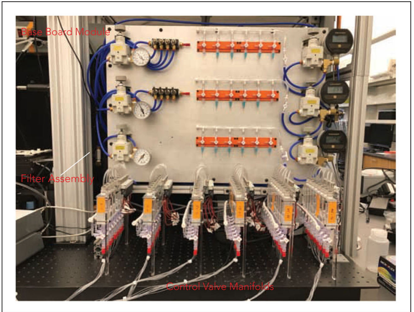
Figure 1. Photograph of a completed pneumatic build (Option 1) with all 5 build modules.
