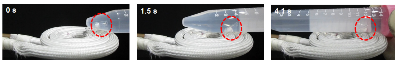
Fig. S11. Related to Fig. 6. (a) Schematic illustrations of utilities of LM/Gel microdevice in digestive organs for advanced drug delivery system, respectively. (b) Sequential snapshots of AMF-induced ( 100 \text{ A m}^{-1} , 245 \text{ kHz} ) relative movement (to the falcon tube) of LM/Gel microdevice (LM 30 \text{ } \mu\text{L} ; 2% w/w agarose 200 \text{ } \mu\text{L} ) in PBS.
