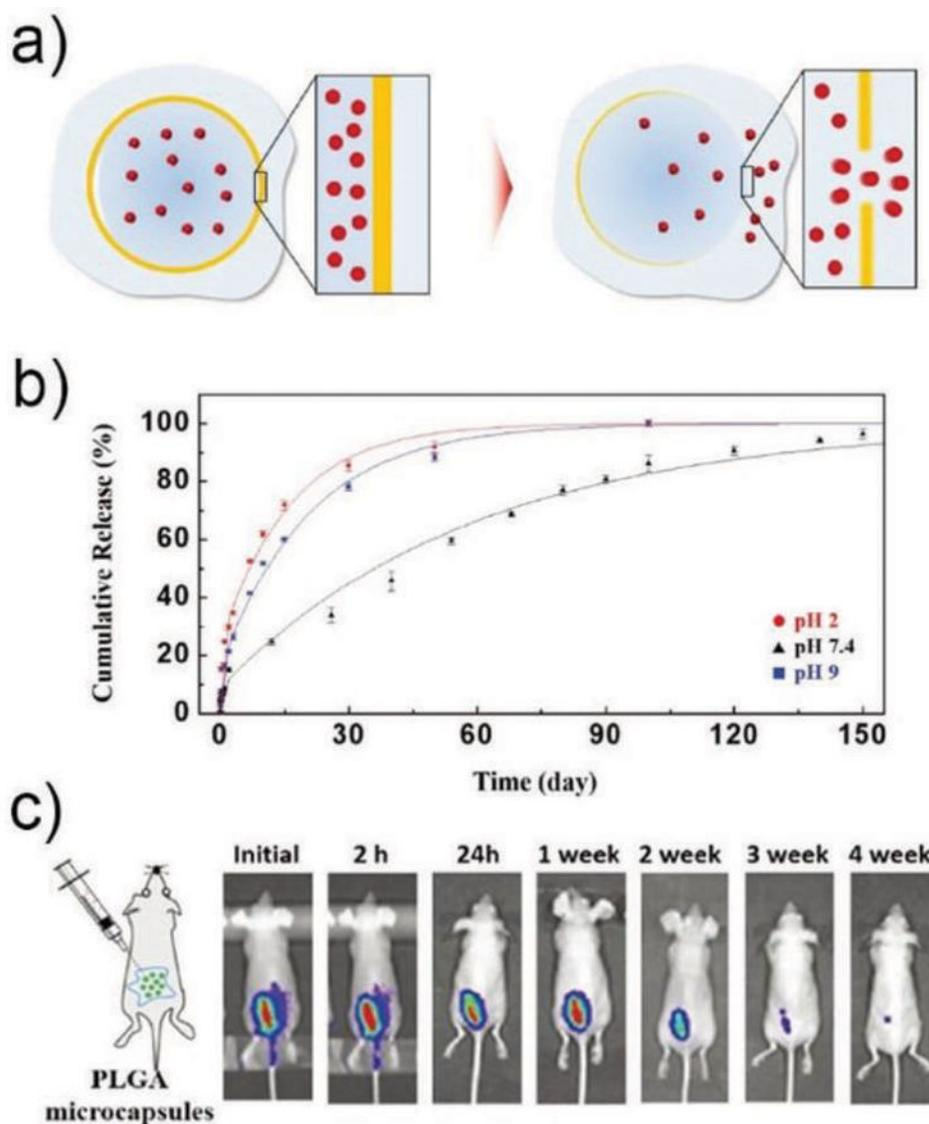
**Fig. 14.** a) Schematic illustration of release of encapsulants through a hole formed at the thinnest part of a PLGA membrane by degradation.<sup>145</sup> b) Cumulative release of sulforhodamine B from the microcapsules at different pH. c) *In vivo* fluorescence images for ICG-loaded PLGA microcapsules that are subcutaneously injected into dorsum of mice. Reprinted with permission from ref. 145. Copyright 2017, John Wiley & Sons, Inc.
