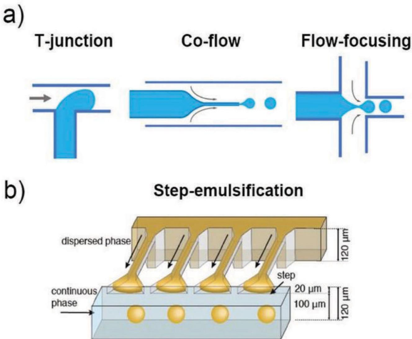
**Fig. 1.** a) Schematic illustration of various channel geometries including cross-flow, co-flow, and flow-focusing. b) Schematic illustration of a step-emulsification channel arranged with four parallelized drop markers.<sup>33</sup> The drop breakup occurs at the step between the nozzle and the continuous phase channel. Reprinted with permission from ref. 33. Copyright 2016, John Wiley & Sons, Inc.
