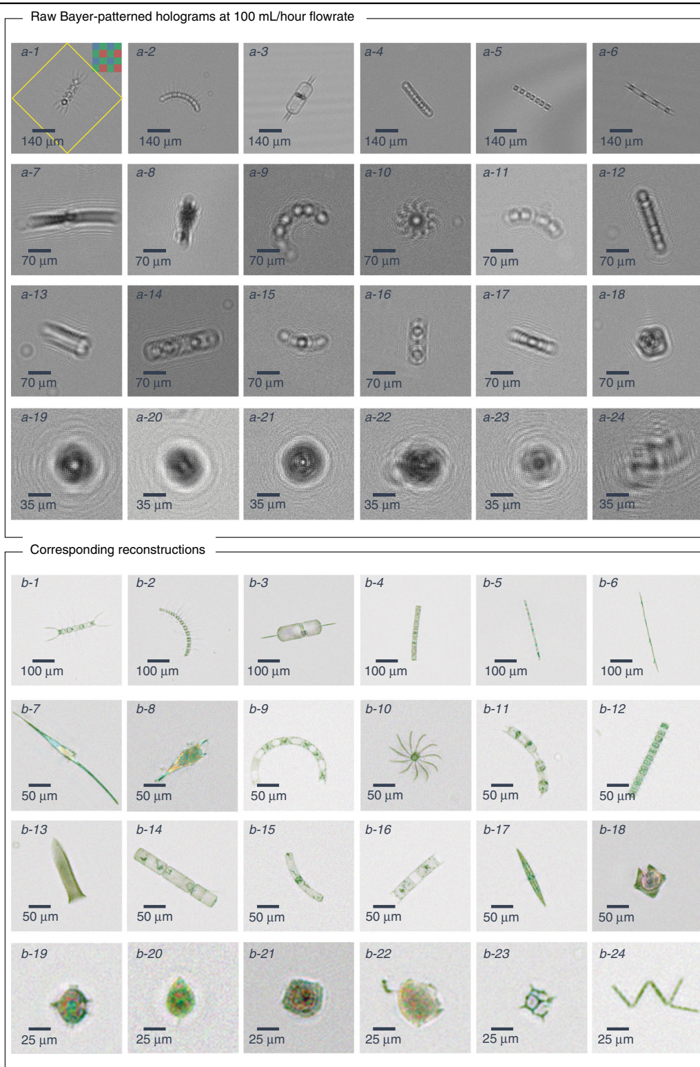
Fig. 2 The image quality of the flow cytometer allows the identification of plankton. Examples of various ocean planktons detected by our imaging flow cytometer at the Los Angeles coastline, represented by their a raw holograms and b phase-contrast reconstructions following phase recovery. The organisms were identified as (1) Chaetoceros lorenzianus , (2) Chaetoceros debilis , (3) Ditylum brightwellii , (4) Lauderia , (5) Leptocylindrus , (6) Pseudo-nitzschia , (7) Ceratium fusus , (8) Ceratium furca , (9) Eucampia cornuta , (10) Bacteriastrum , (11) Hemiaulus , (12) Skeletonema , (13) Ciliate , (14) Cerataulina , (15) Guinardia striata , (16) Lithodesmium , (17) Pleurosigma , (18) Protoperidinium claudicans , (19) Protoperidinium steinii , (20) Prorocentrum micans , (21) Lingulodinium polyedra , (22) Dinophysis , (23) Dictyocha fibula (silica skeleton), and (24) Thalassionema . The yellow rectangle in a-1 represents the segmented and 45° rotated area corresponding to the reconstructed images
