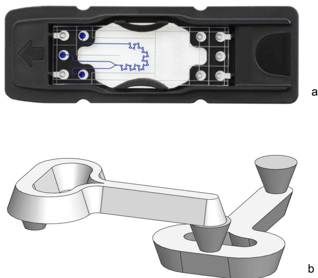
Figure 3. Mixer chip: (a) Layout of the mounted teardrop mixer chip (45 mm long, 15 mm wide). (b) Enlarged view of the teardrop mixing element. Channel width is 150\text{--}200 \mu\text{m} , and the channel depth is 150 \mu\text{m} . The mixer chip is produced from borosilicate glass, using negative dry film resist and powder blasting.
