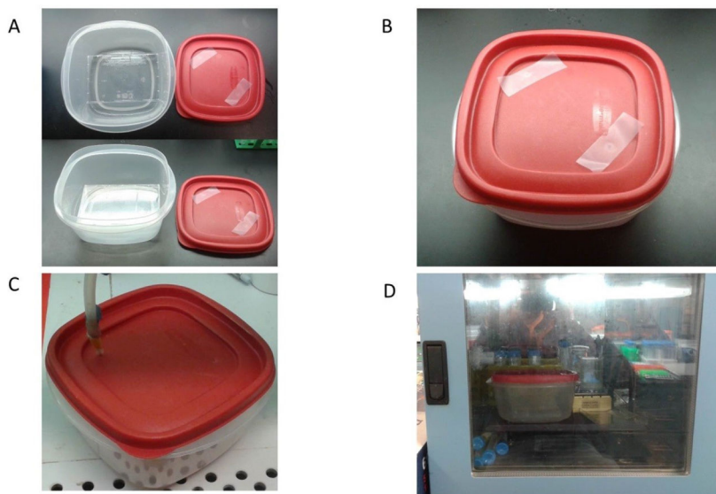
Figure 7. Tupperware enclosure setup for nitrogen perfusion and gelling of ExFISH cultured cell samples. (A) Open Tupperware with a plastic platform for supporting the sample and a pool of water at the bottom for humidity. (B) Closed Tupperware with two inlets on the cover sealed with tape. (C) Nitrogen perfusion of sample inside the Tupperware. Tape seals have been removed and a nitrogen line has been inserted through one inlet, with the other remaining open to allow air to escape. (D) Following nitrogen perfusion, the two inlets are sealed with tape, and the Tupperware containing the sample to be gelled is placed in a 60°C incubator.
