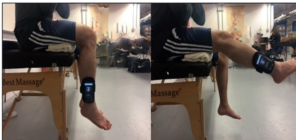
Figure 4. Knee joint position sense (JPS) measurement using iPod touch device (Apple Inc., Cupertino, CA, USA) integrated with custom-made application software.
