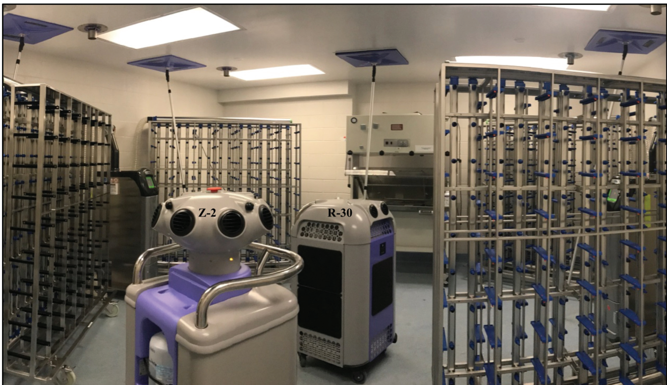
Figure 3. The flex room where assembled IVC racks connected to AHU were VHP exposed in the active–closed setting, with AHU set to the VHP cycle, during months 6 through 12. All equipment required for a scheduled housing room change-out in its entirety was VHP decontaminated the day before by using the Z2 generator and R30 accelerator. Other portable equipment (here, an animal transfer station with its work surface propped open) was VHP decontaminated in the flex room also.
