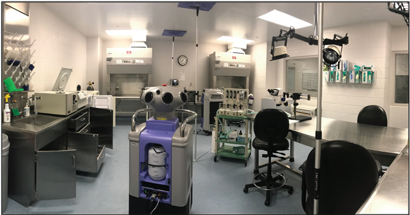
Figure 5. Procedure rooms were VHP decontaminated with all supplies and equipment present, centrifuges open, biologic safety cabinet sashes raised, anesthesia induction boxes open, and all casework drawers and shelving exposed.
